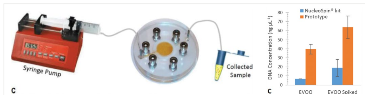
Figure 5. Experimental set up for DNA extraction experiments and average DNA concentration of elution samples obtained from extra virgin olive oil (EVOO) samples DNA-spiked and non-spiked with the commercial NucleoSpin® kit versus the results obtained in our prototype from the same samples. From: Anal. Chim. Acta. 1020 (2018) 30–40. doi:10.1016/j.aca.2018.02.079).
