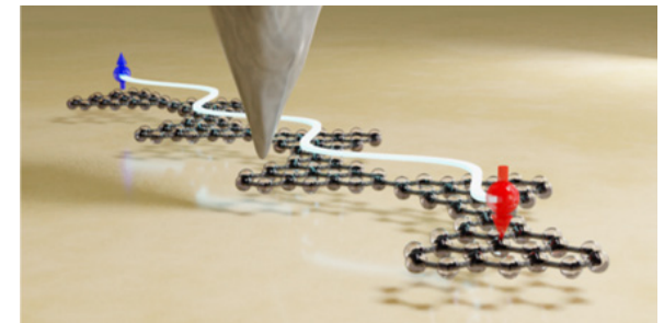
Artistic rendering of a triangulene quantum spin chain adsorbed on a gold surface and probed with the sharp tip of a scanning tunneling microscope. While each triangulene unit has a total spin of 1, quantum correlations in the chain lead to spin fractionalization, such that the terminal triangulene units exhibit a spin of 1/2. Image: Empa
