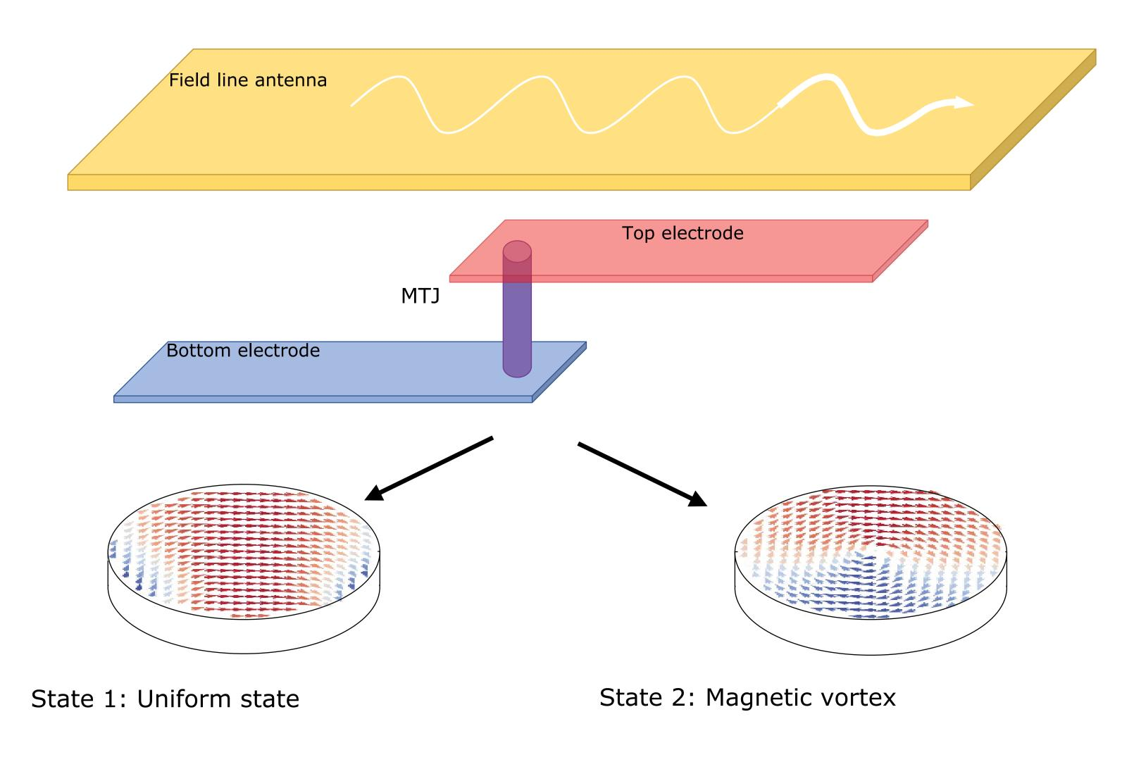
Due to the nanosize of the individual devices (~100 nm device diameter), there is a clear possibility for scalability, with multiple devices being connected to a single field line antenna producing synchronised but uncoupled random bits. www.inl.int
